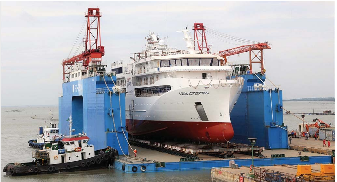
CORAL ADVENTURER, as she will look upon her debut in Australian waters on April 24, 2019 (top). She is currently fitting out in a floating drydock at Vard Vung Tau Shipyard in Vietnam (bottom). (Coral Expeditions)
